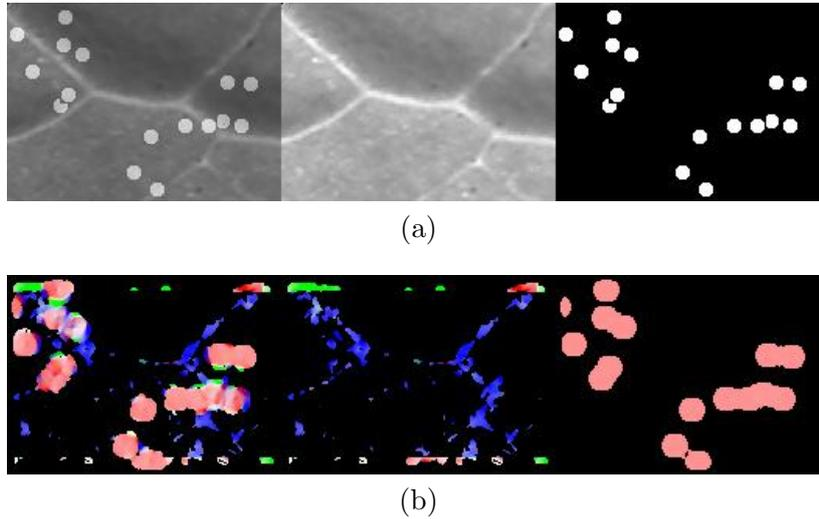
**Figure 4.9:** (L-R)Frames from synthetic heart sequence, "heart-wall" extracted using median filtering, "RBCs" extracted using subtraction method. (a) Frames as got from the algorithm. (b) Flow-maps in DC format got after flow analysis.
