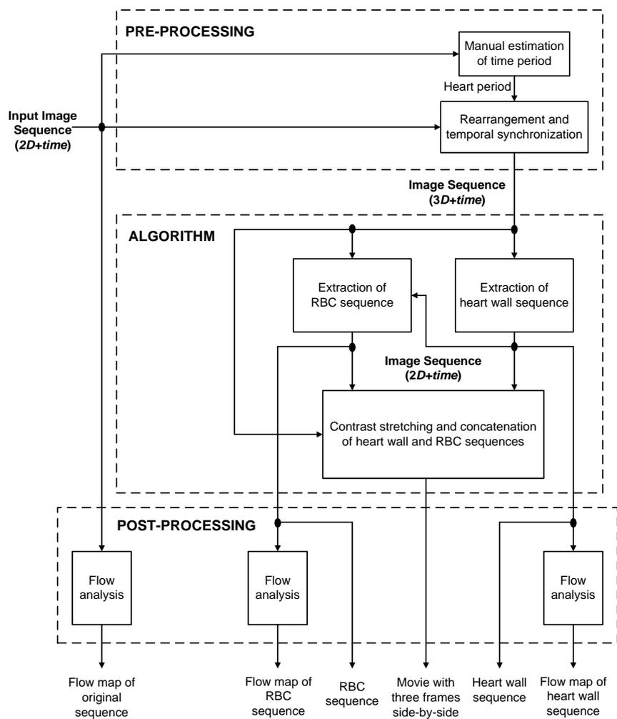
**Figure 2.1:** Top-level block diagram. The dotted boxes indicate the various stages of the algorithm.
